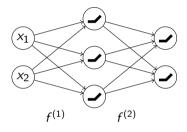
▶ A ReLU network computes a continuous piecewise linear (CPWL) function:  $f = f^{(\ell+1)} \circ f^{(\ell)} \circ \cdots \circ f^{(1)}$  where  $f^{(i)}$  is a ReLU layer for  $i \in [\ell]$
