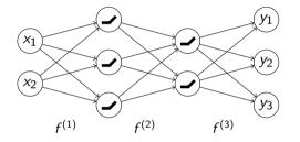
A ReLU network computes a continuous piecewise linear (CPWL) function:  $f = f^{(\ell+1)} \circ f^{(\ell)} \circ \cdots \circ f^{(1)}$  where  $f^{(i)}$  is a ReLU layer for  $i \in [\ell]$  and  $f^{(\ell+1)}$  is the affine linear output layer.
